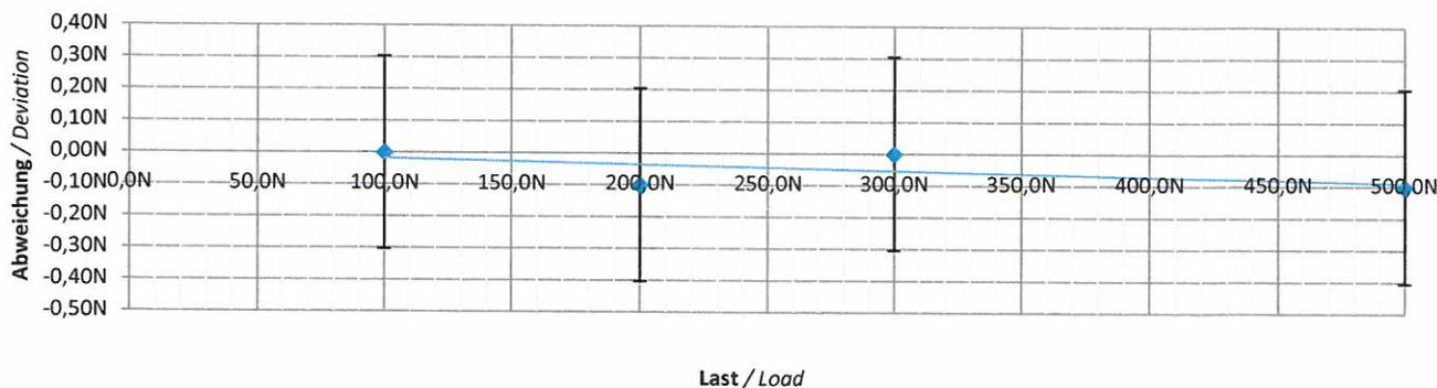
Messergebnisse (Druckkraft) / Measurement results (compressive force)
