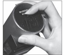
The battery box is located on the bottom of the tester. Open the box by pushing the locking lever over the battery symbol as shown in the picture (see image) and replace the battery.
